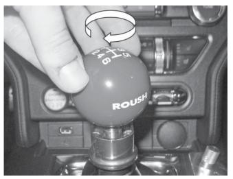
3. Screw the shift ball down until the bottom of the ball sits lower than the top of the positive lockout, and then continue to turn clockwise until the shift pattern on the top of the ball rests in the desired position.
