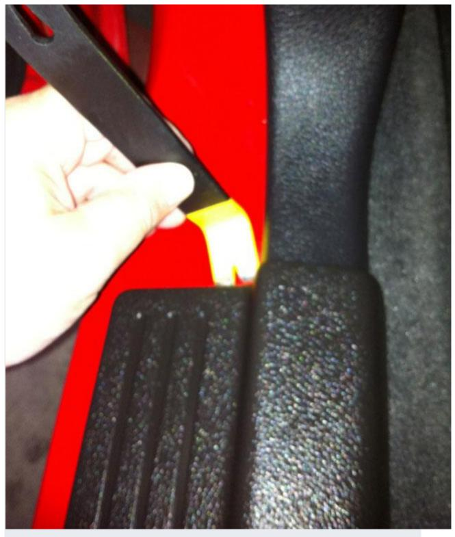
4. Remove the small plastic clip on the driver's side kick panel. Then, carefully remove the plastic side kick panel by pulling back towards the rear of the vehicle.
