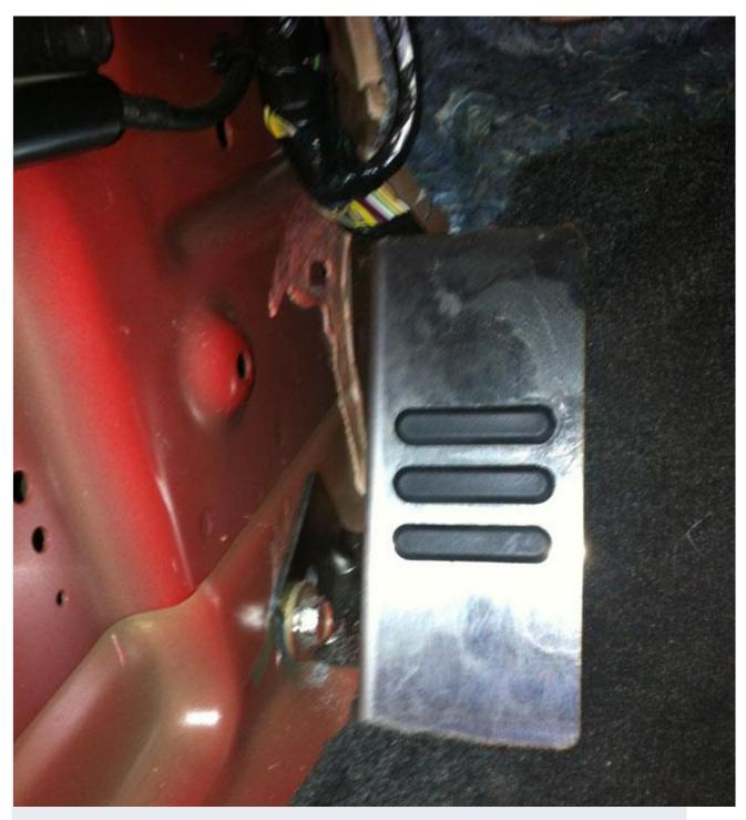
8. Reinstall the kick panel and the trim piece that secures it. If your vehicle is equipped with an alarm override button, carefully reinstall the ring nut and washer that secure the button to the plastic kick panel. Reinstall the small plastic clip on the driver's side kick panel.
