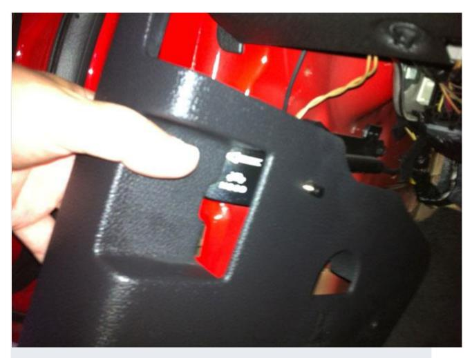
5. Locate and loosen the bolt on the side of the body using a 13mm socket. Do not remove this bolt. Simply loosen it enough to slide the new CDC dead pedal in behind it, which should be about 1/2 inch. Note: Be careful of the wiring harness near this bolt. You may have to remove the plastic mount that connects the wiring harness to the chassis in order to move the wiring harness aside.
