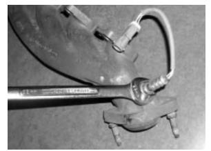
Removing the oxygen sensor.
