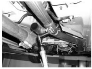
Separate H-pipe from tail pipe.
