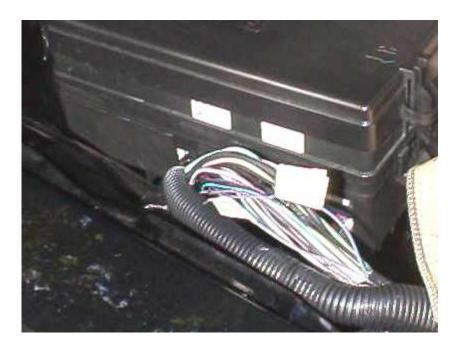
2) Open wire loom "A" (if necessary, remove or carefully cut any electrical tape to
