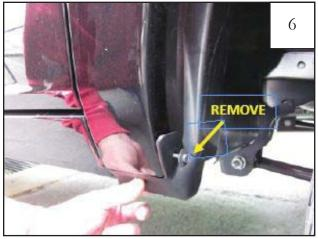
Models with Stone Guards Only (Optional): If you encounter a fit problem, remove chip guard at bottom rear of wheel well. Remove screws using an 8mm socket
