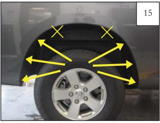
Remove these six factory installed screws using an 8mm socket wrench. X's indicate a factory screw that will not be removed.
