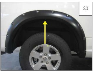
Start Screw (SW1-0056) using a Phillips Head Screwdriver. *Do not tighten*.
