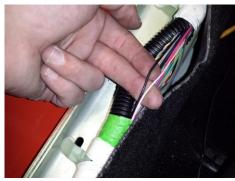
Step 4: Locate the wiring harness that runs down each door sill and expose the wires within.
