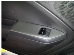
Step 5: Pull the window control assembly towards the interior of the vehicle to remove it.
