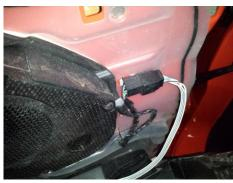
Step 10: Unplug all connectors holding the panel to the door leaving the door handle cable attached.
