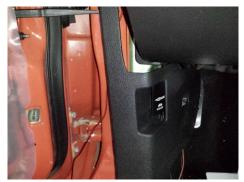
Step 2: Remove the interior kick panels and door sill panels.
