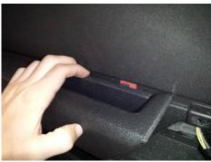
Step 7: Using your fingers or interior trim removal tools, pull the panel behind the door pull out and up to remove it from the vehicle.
