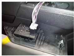
Step 6: Disconnect the wiring harness connected to the window switches and remove the 7mm screw behind it from the vehicle.
