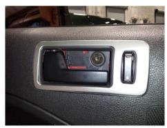
Step 4: Pull the inner door handle out and pop the inner cover out exposing the torx screw below.
