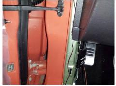
Step 3: Using a stiff wire tool, route the tool into the harness to pull the wires into the interior of the vehicle.
