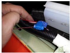
Step 5: Wire the mirrors into the vehicles harness using the supplied wire splices.
