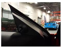
Step 1: Remove the driver's side mirror control panel by pulling away from the door
