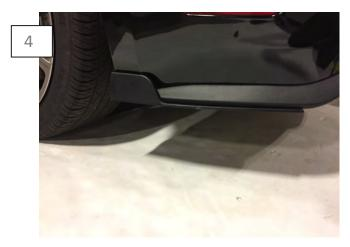
Install the winglet using the factory push clips. \*\*Note: There are a tight fit but they will press all the way in. Apply firm even pressure to the taped surface to ensure proper adhesion.
