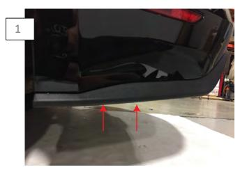
Front under the vehicle, remove the (2) bumper push clips. \*\*Note: These clips will be reused. Thoroughly clean the bottom edge of the bumper trim to remove any and all wax/grease. \*\*Note: Use isopropyl alcohol to ensure the cleanest possible tape surface.
