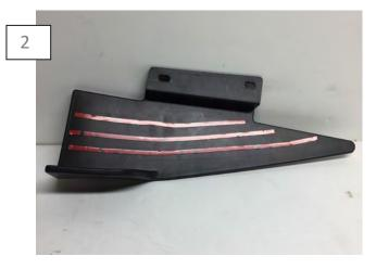
Apply 3M tape the to winglet surface as shown above.
