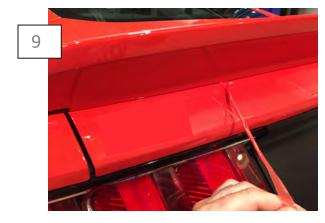
With a helper, start each of the (4) screws to hold the spoiler in place. Once the spoiler is loosely mounted, peel the tape backing off as see above. Then tighten the screws the rest of the way.
