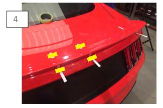
Test fit the spoiler, center it on the back edge of the deck lid. Securely tape the templates to the deck lid where they lay. Carefully remove the spoiler from the templates. \*\*Note: This is the most important step to ensure the the holes are drilled in the correct location.
