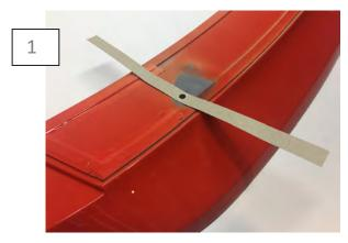
Using the provided drill template. Remove the center adhesive backing. Place the adhesive side on the spoiler, centering it over the bolt hole.
