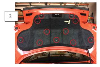
To remove the interior decklid cover panel, remove the (9) push pins and unscrew the (2) rubber bumpers. Manipulate the cover around the latch to remove it from the vehicle. Then remove the deck lid plugs located top left and right of the panel.
