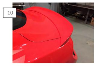
Apply firm even pressure to taped surfaced to ensure proper adhesion.
