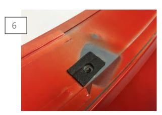
Place the supplied foam pads over the mounting holes on the spoiler. Trim as needed.
