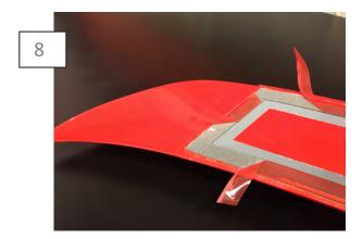
Peel back the first two inches of the tape backing from each end of the tape strips. \*\*Note: Do not peel the tape back all the way off just yet.
