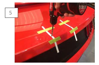
Once the spoiler is removed, carefully drill the center of the template holes. Finish with a 7/32 drill bit. \*\*Note: Use touch up paint to cover any exposed metal to prevent rusting.
