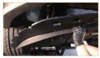
**2.** Remove the eight pop clips that hold the plastic air diversion cover in place. Remove the cover.
