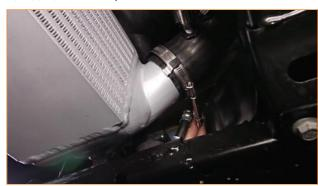
**29.** Tighten the worm-gear clamp on the cold-side pipe. Make sure that the boot is seated all the way on the intercooler. (7mm socket, 7mm socket wrench, or flathead screwdriver)
