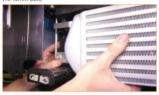
**27.** Install the supplied set screw on the driver side. (1x M4 x 0.7 x 12mm button-head bolt, 1x M4 lock washer, 2.5mm Allen key)
