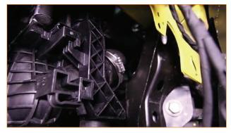
**14.** Loosen the worm-gear clamp on the hot-side pipe connecting to the intercooler. (7mm socket, 7mm socket wrench, or flathead screwdriver)
