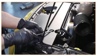
**3.** Remove the bumper hardware, but do not fully remove the front bumper. (4x pop clips and 6x 8mm screws)
