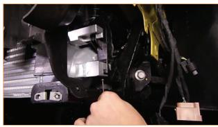
**28.** Tighten the worm-gear clamp on the hot-side pipe. Make sure that the boot is seated all the way on the intercooler. (7mm socket, 7mm socket wrench, or flathead screwdriver)
