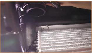
**16.** Remove the plastic cover from the side of the intercooler and rotate to the side.
