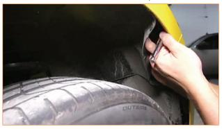
**5.** Unclip the bumper from the vehicle by pulling the side corners out first, and then lifting the top holes up off the pegs. Once the bumper is loose, unclip the six wire harnesses for the turn signals, headlights, and fog lights. Remove the bumper.
