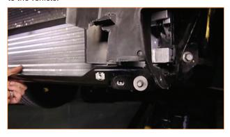
**35.** Reattach the air shutters. Make sure to route the air shutter arm around the front crash beam. The air shutter arm will reattach to the clip on the front air dam. (2x pop clips, 4x 8mm bolts)
