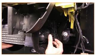
**20.** Lift the intercooler hangers up while pulling forward toward the front of the vehicle.
