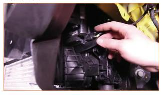
**13.** Loosen the worm-gear clamp on the cold-side pipe connecting to the intercooler. (7mm socket, 7mm socket wrench, or flathead screwdriver)
