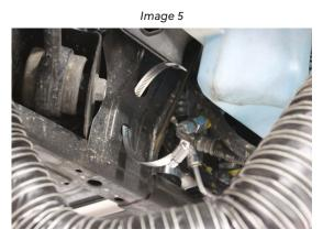
Step 28) Test to ensure the tubing does not bind or pull on the clamps by turning the wheel all the way to the left, then all the way to the right. If binding or pulling happens, adjust the routing, re-secure tubing, and re-test. Each side.
