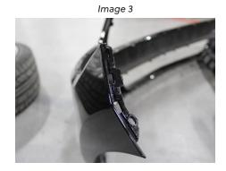
Step 11) Remove the fog lamp/turn signal housing from the backside of the facia by removing the (6) 7mm bolts (see image 4). (2) of these have washers. Note the location where these (2) were removed from as they will need to go back to those same locations. Now, using a flat head screwdriver, release the tabs that hold the housing in place, starting at the outside tabs and working your way in. Each side.
