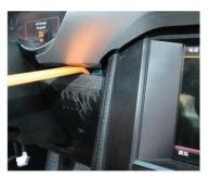
Use the provided trim removal tool(s) to pry open the center dashboard trim. There are 4 clips holding the trim piece to the console. All 4 clips are located towards the front of the panel. Check where the clips are located from the new HUD unit to understand the structure underneath. **Note:** The center air vent trim do not need to be removed.
