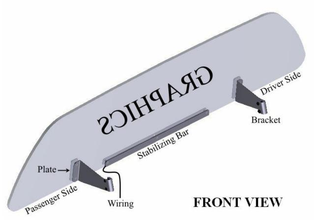
"Note: This wind deflector is installed by attaching the two mounting brackets to the factory designed front seat headrest posts so that the glass is to the rear of the headrest.
