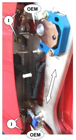
8.) Adjust the **height** of the door by moving the chassis plate vertically. You might have to loosen bolts **(L)** on the chassis plate to do this.
