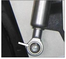
16.) Carefully pivot the door up, place in the gas damper (P) on the according mounting point on the chassis plate. Secure it with the supplied security ring.
