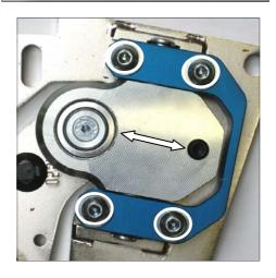
7.) Attach the swing arm to the chassis plate with the 4 included Allen bolts and adjust the door via moving the swing arm to chassis plate adjustable (2) connection mount with horizontal door gap adjuster (2) in the right or left direction until gap measurement is like original.
