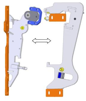
1.) Disassemble the swing arm (N) off the chassis plate (O).
