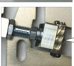
6.) Position the lower adjustment screw (1) in that way, which the door closes in the center position.
