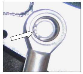
15.) Hang in the gas damper (P) on the fitting point of the swing arm. Secure it with the supplied security ring, by means of needlenosed pliers.
