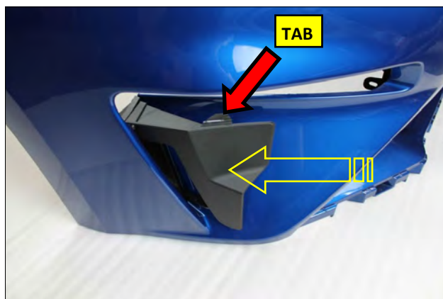
24. Slide the RTR Turning Vane mounting posts into the RTR Bumper Vent and remove the adhesive backing from the mounting tab.
