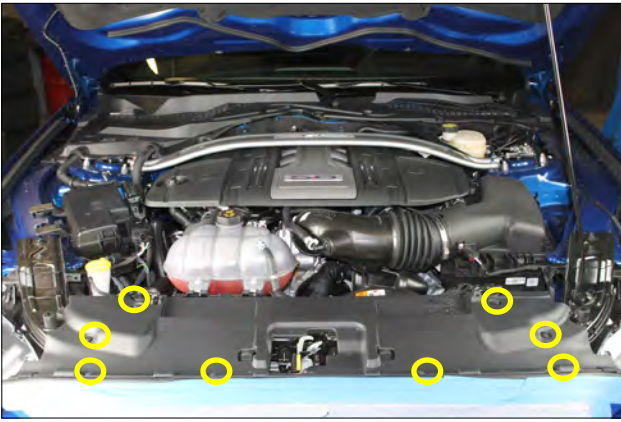
29. With the help of an assistant, lift the bumper cover back onto the vehicle and secure it using the OEM hardware. Reinstall the core support cover using the plastic rivets.
