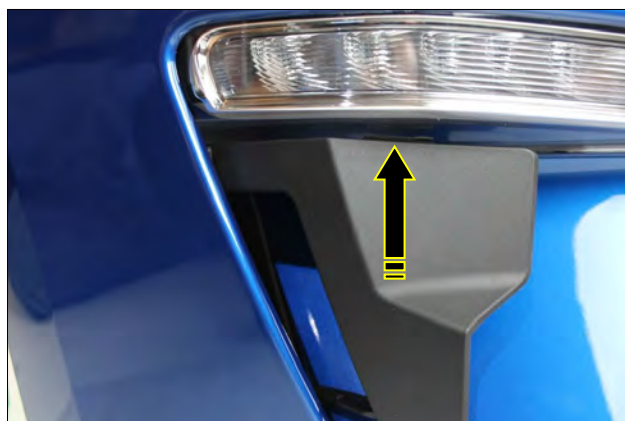
28. Press firmly under the mounting tab until it contacts the underside of the accessory lamp and bonds. Repeat steps 18-27 on the opposite side of the bumper cover.
