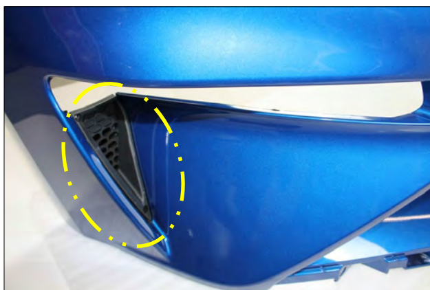
23. Inspect the RTR Bumper Vent installation from the front of the bumper cover assembly and confirm all tabs are fully seated.
