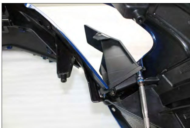
25. Secure the RTR Turning Vane to the RTR Bumper Vent using three of the supplied 5mm Screws.
