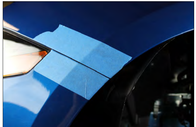
8. RTR recommends using painters tape as protection for areas susceptible to abrasion during disassembly and assembly.
