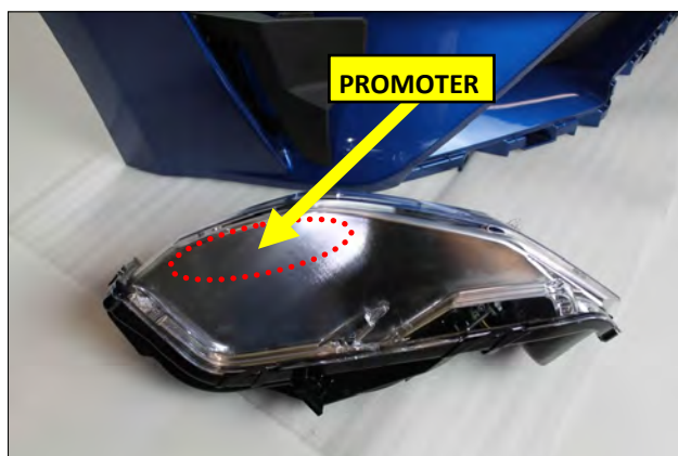
26. Wash the accessory lamp using a mild soap and water solution. When completely dry, prep the area shown using the supplied Adhesion Promoter.
