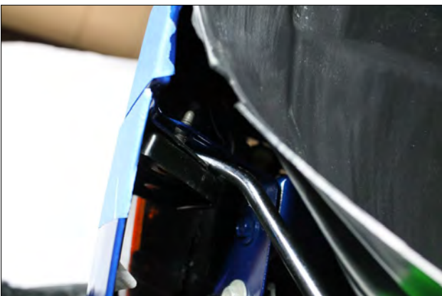
9. Using a panel tool or equivalent, pry the stud blocks away from the bumper support.
