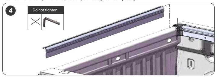
4. Slide front rail assembly by inserting L bracket into T-slot, do not tighten set screws.
