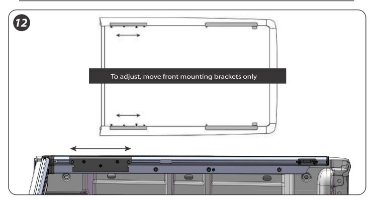
12. With your cover closed, take a quick inspection to make sure that the cover is sitting square to the Tango Track. To adjust the cover front to back evenly, move both of the front mounting brackets forward or rearward accordingly. To adjust to one side or the other, move the front mounting brackets forward or rearward independently.
