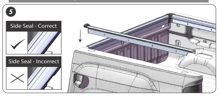
5. Slide the left rail assembly in place by inserting the L bracket in to the T-slot, do not tighten Note: Lift up on the front rail assembly to create enough room to insert the L bracket into the T-slot. *Note: Be sure side rubber is not pinched under rail assembly.*
