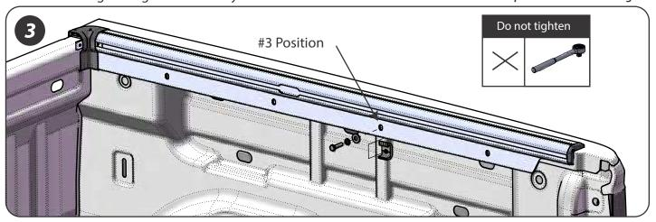
3. Install one clamp in the #3 position, do not tighten completely.
