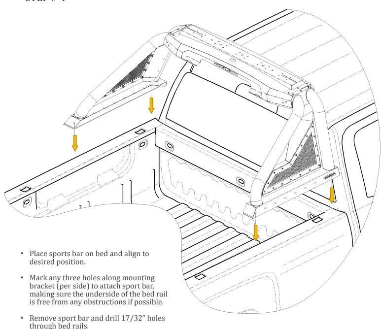
• If holes can not be drill through top and bottom of bed rail proceed to step #4.1.
