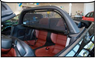
There are 4 straps that hold your wind deflector down. Two use the child anchor system and two attached to the to bottom of the trim panel
