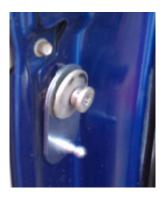
Tighten the bolt with the T45.
