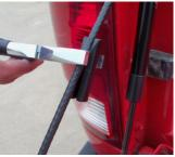
Failure to remove the limiter and to install the cable clip will cause the cable to bind or become caught between the shock and truck bed. This may lead to vehicle damage, so these steps MUST be done.
