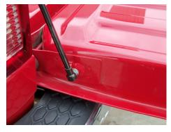
Periodically check the upper and lower mounting locations to insure that parts have not loosened through repeated use. If either mounting location is found to be loose, re-tighten the hardware as needed.
