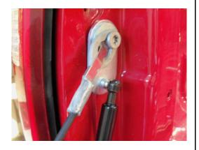
Install the narrow end of the shock on the ball mount .
