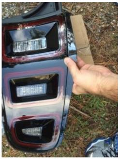
5. With the trim applied to the tail light, feed the tail light connector through the pass-thru and gently press on the rubber grommet around the wiring to allow the channel to seal with the pass-thru.
