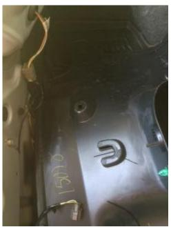
4. Push the release tab on the tail light wiring harness and unplug the connector from the socket.
