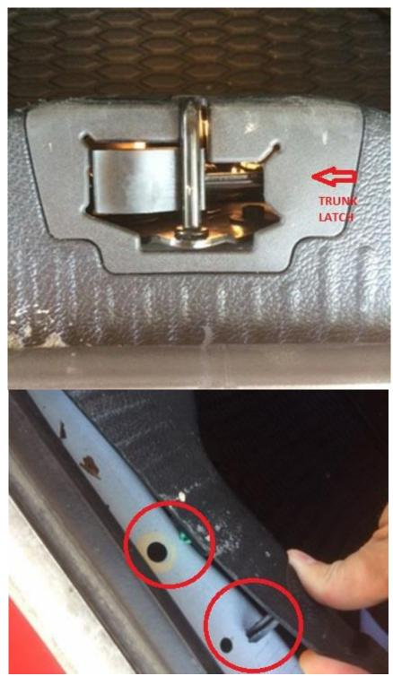
3. Lay down the trunk latch trim cover. Be careful not to pull on the trunk light wiring harness.
