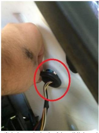
6. Locate the three (3) bolts on the back of the tail light and guide them through the three (3) holes in the car body until the tail light is firmly in place.
