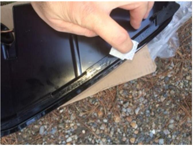
3. Remove the three (3) red 3M tape backings on the Raxiom Tail Light Conversion Trim to expose the adhesive side of the tape.
