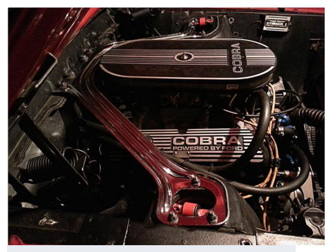
6. With the car on the ground, we removed the nuts that hold the export brace to the Mustang shock tower, re-fitted the shock tower tops, tightened every nut for the final time and screwed down the shocks to the caps.
