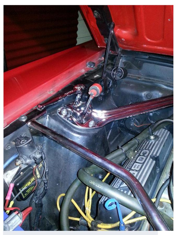
7. Tighten up all the fender bolts and you've completed the installation of your new Mustang Scott Drake Export Brace.
