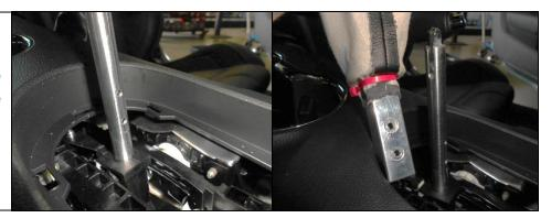
11. With the shift boot still inverted slide the Hurst pistol grip down over the lower stick and secure it in place using the two provided set screws.
