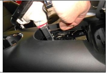
12. Put the shifter back into the Park position. Plug the wire harness back into the shift indicator and snap it back into place.
