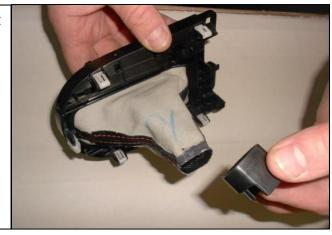
8. With the shift boot inverted, orientate the Hurst pistol grip handle in the correct position and slide it through the boot as far as it will go.
