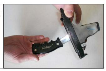
9. Zip tie the shift boot to the pistol grip. There is a groove machined into the handle that is intended for the zip tie to lock into.
