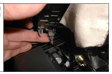
**CAUTION:** With the engine off, the emergency brake set and the front and rear wheels blocked, move the shift handle back far enough to gain access to the two Philips screws that bolt the shift handle to the lower stick.
