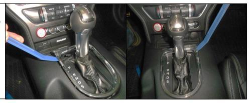
2. Starting from the front of the shift indicator, pry up to release the forward locking clips. Then work your way down the side to release the remaining ones.
