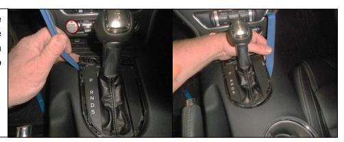
3. Raise the shift indicator high enough to unplug the wire harness from the bottom of the shift indicator.
