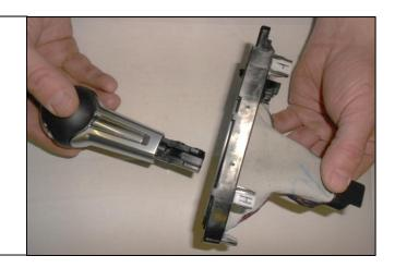
7. The shift boot ring is glued to the shift boot and must be removed. Carefully peel the two apart. The ring will not be used moving forward.
