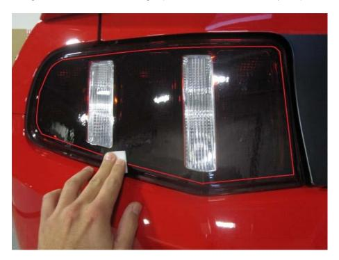
**Step 2:**Peel the backing from the 3M tape as shown below.
